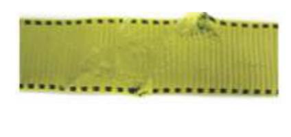
Discoloration and brittle or Stiff area due to Chemical or Ultraviolet sunlight damage
