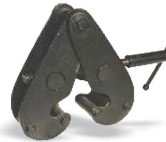
Versatile jaws designed to mount on a wide range of tapered or flat beams. Built-in suspension bar allows for low headroom. Easily installed and adjusted by hand. Provides temporary or permanent mounting point for hook mounted hoists or lever pullers. Designed to minimize stress applied to beam. Range from 1 Tons to 5 Tons. Large Capacities available on request.
