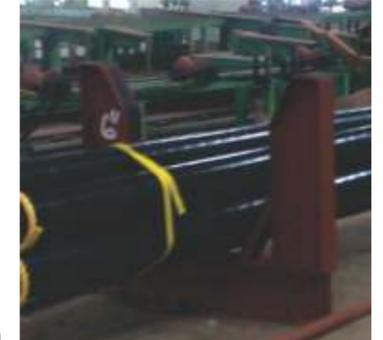
The pipes have to be stacked in fixtures/ steel frames so that initial shape is made by the pipes in form of hexagonal bundles. As shown in pictures above, single stand or multiple stands near packing/exit area will facilitate the bundling. These frames can be fabricated considering diameter of pipe and number of pipes in one bundle. For coated pipe the frames should be properly coated /covered by PU Elastomer/ foam/Rubber Sheet or any suitable material to avoid scratches.
