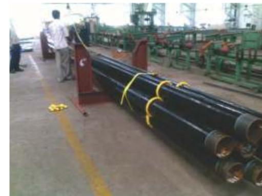
For coated pipe, buckles will also be coated so that no scratches will be on pipes. Process of lashing is illustrated as below
