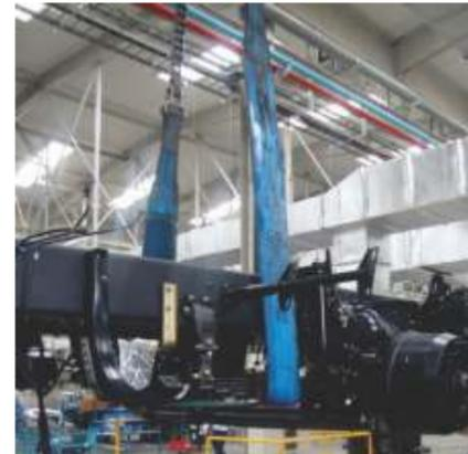
Now all your turning devices for turning automobiles, chassis, Marble Blocks, Machines, Moulds infact, rather anything can be secured on our range of Ferretero ROTOMAXX slings. These are heavy duty slings impregnated with Polyurethane and plasticized coating to grip the load and are almost Anti-cut. These slings can be made up to 30 ton load turning.
