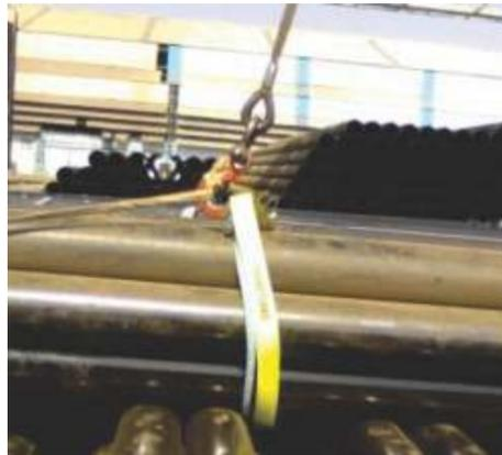
Pre-slung endless slings/One Way Slings are inserted in pipe bundles, which are now ready to dispatch.
