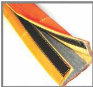
The description of Dynaflexx sleeves need to come under - Another Innovation is Dynaflexx. Cut resistant Kevlar/HMPE sheet stitched with Velcro. Most efficient in low temperatures and can lift products with protruding sharp points, weld spats. This sleeve provides cushion and protection both. The sleeve allows sling to slide in freely providing maximum wear resistance.
