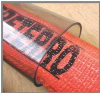
Polyurethane blended sleeve upto 30 tons capacity. Clear construction to view damages to webbing. Side stitches with triple AA on stitches for extra long life.
