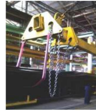
Uses Anti-Abrasive, Anti-cut sleeves to protect round slings from damage by sharp edges, we have wide range of protection sleeves. (See Sling Protection).
