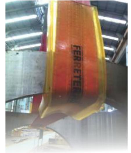
FERRETEXX is Extreme condition sleeve to lift almost anything. Sharp coils, Ultra sharp edges are now easiest job for synthetic slings. Available in both Round slings and Flat webbing slings for loads upto 300 tons. These sleeves stick to the job and are extremely cut resistant. To be used for super sharp cut edges.
