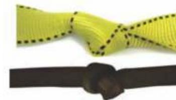
Sling Weld Splatters and Charring/Melting
